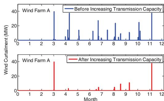
Figure 6. Wind curtailment in wind farm A before and after increasing the transmission capacity
