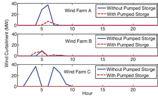
Figure 3. Wind curtailment in three wind farms for the 6<sup>th</sup> day in selected two weeks
