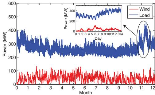
Figure 2. Wind and load profiles for the whole year
